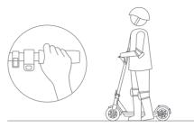
DO NOT press the throttle when walking with the scooter.
